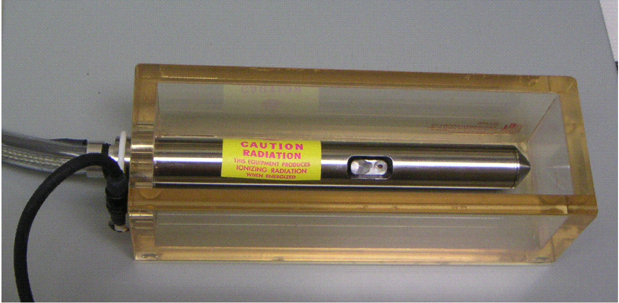
Figure 2. Probe in Radiation Enclosure with Interlocks
