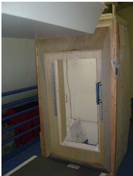
Figure 12. CQ low-fidelity wood mock-up with preliminary component layout.
