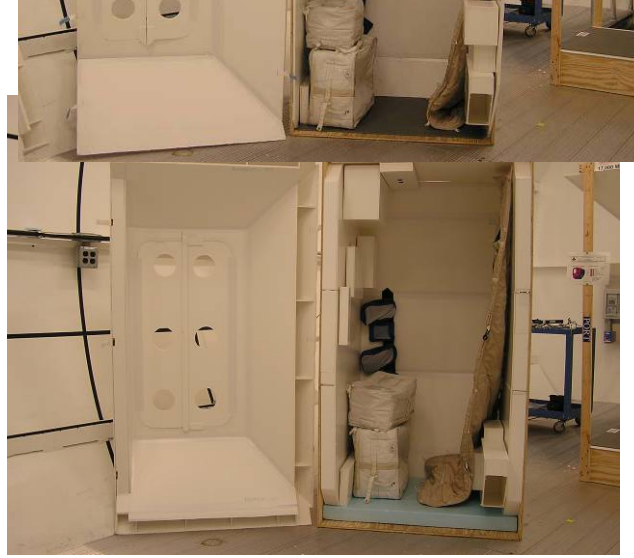
Figure 11. CQ volumetric foam mock-up with 7.6 cm thick walls for radiation protection shown.
