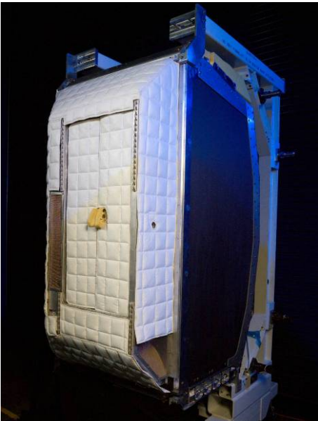
Figure 13. External of CQ mid-fidelity mockup on rack handling assembly.
