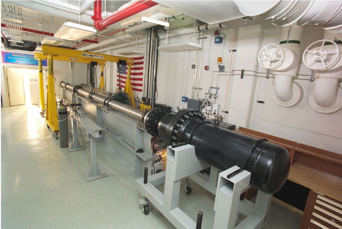
Figure 3. Gas Gun Used for Ballistic Impact Testing
