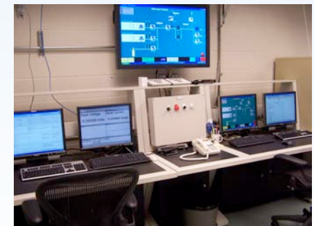
Fuel Cell Testing Laboratory 3 test cells capable of testing complete fuel cell, electrolyzer and regenerative systems up to 25kW
