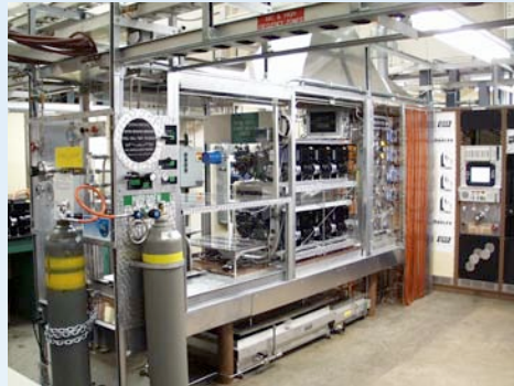
Hydrogen/Air Fuel Cell Test Facility Stack and subsystem testing up to 12 kW (Can be modified for other fuels)
