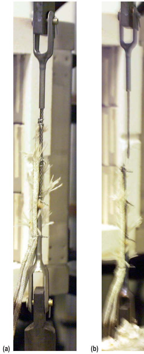
Figure 31. 5369-ELV-9 (a) before testing and (b) after testing.
