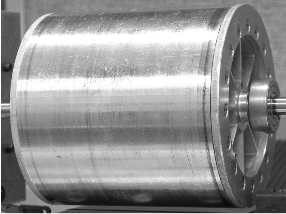
Figure 10.—Four inch radial Halbach magnetic bearing rotor.
