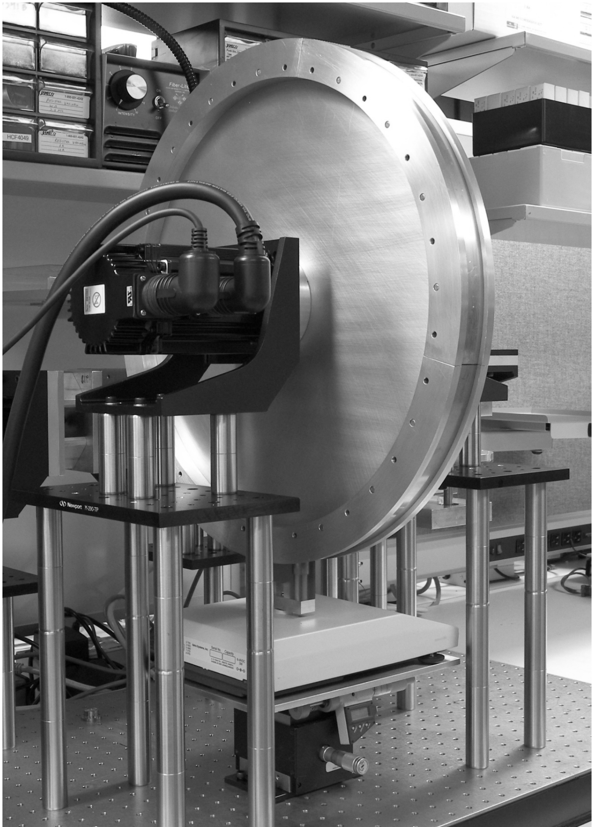
Figure 4.—Twenty inch rotor characterization hardware setup.
