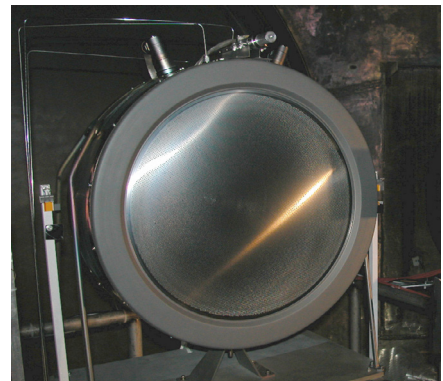
Figure 1. —NEXT EM1 ion thruster mounted in VF6 at NASA GRC for wear testing.
