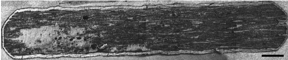
Figure 13. Polished cross-section of C/SiC composite coupon after exposure at 816°C in flowing (100 ccm) 0.5 atm O 2 for 25h. Note complete oxidation of T-300 fibers. Scale = 0.1 cm.
