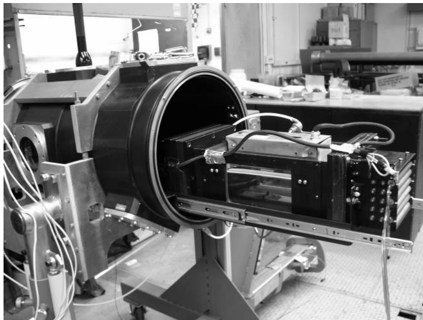
Figure 2. Photograph of the FIST tunnel in the containment chamber.
