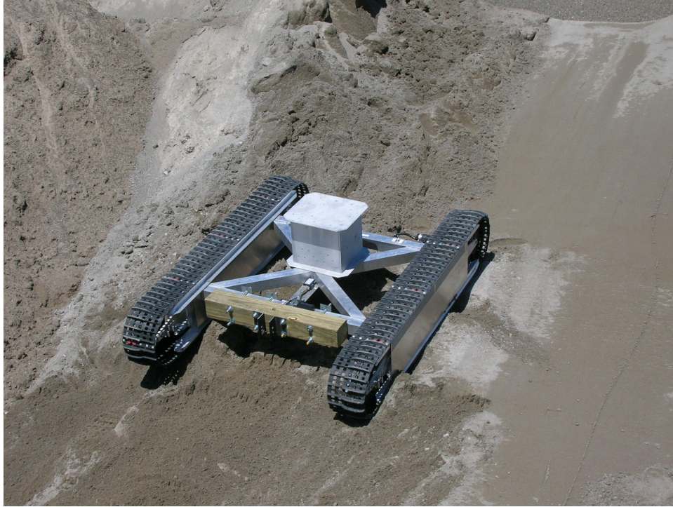
Figure 5.—The simulator mounted on the Carnegie Mellon University Highlander rover platform.
