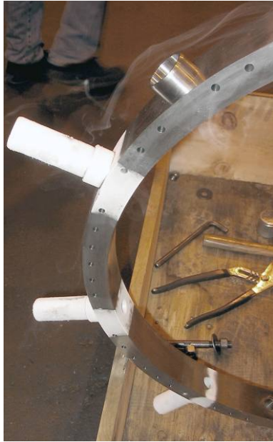
Figure 9.—Photograph showing frost on the new test chamber outer wall just after the shrink fit installation of an actuator support tube.
