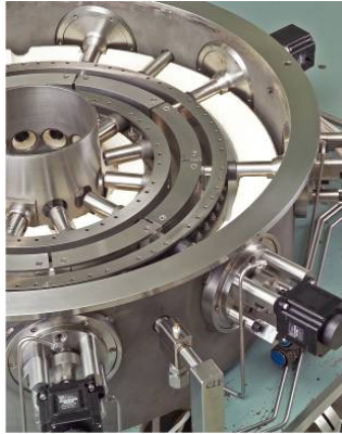
Figure 2.—Photograph of the active clearance control system.
