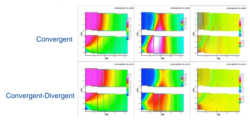
C-D nozzle extends potential core, reduces TKE, 'reduces' shocks.
