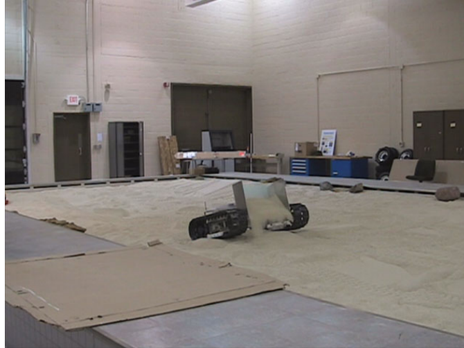
Figure 1. Cratos building a small ramp.
