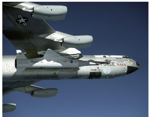
Figure 8 Hyper-X stack being carried to altitude by the NASA B-52B
