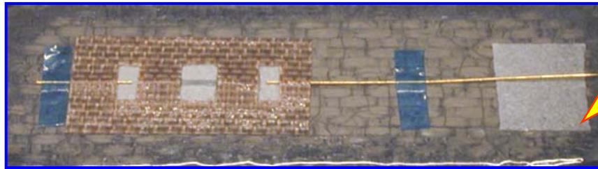
Flame-spray sensor attachment
