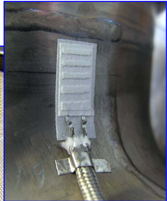
Spot weld three-conductor leadwire
