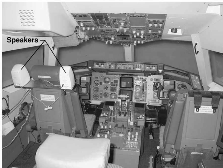
Figure 2. Interior view of Langley IFD simulation cockpit. (Stereo) speakers were designed to provide a lateral acceleration cue.
