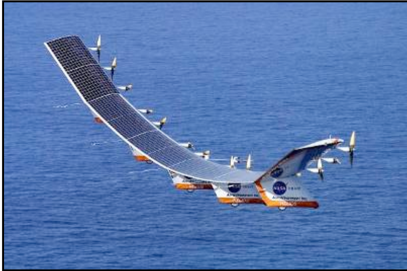
Helios wing dihedral on takeoff
