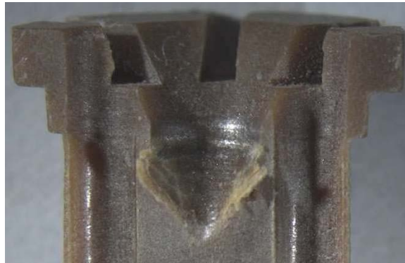
Figure 11. Split Spool Deformation
