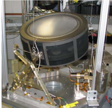
Figure 6.—Gimbal Assembly and PM Thruster undergoing Articulation Testing at JPL.
