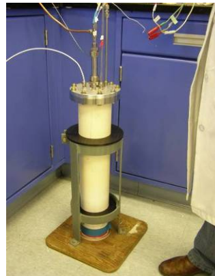
Low-Temperature Electrolysis Cell at KSC
