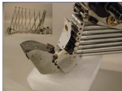
Surveyor Arm/Scoop Re-fabrication and Controlled Laboratory Testing at GRC
