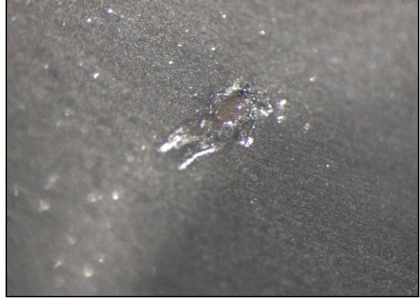
Fig. 6. Irregularly shaped gouge on aluminum kidney surface.
