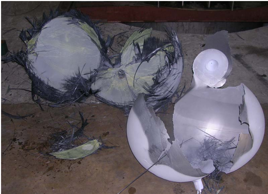
Figure 7. Cryogenic Burst Test for Part No. D4970, S/N 002
