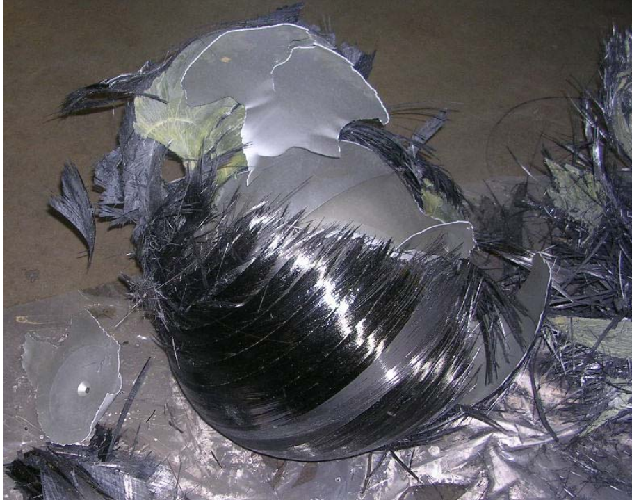
Figure 8. Ambient Burst Test for Part No. D4971, S/N 003
