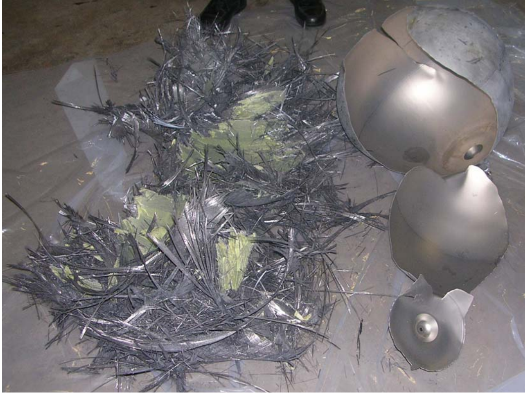
Figure 6. Ambient Burst Test for Part No. D4970, S/N 006
