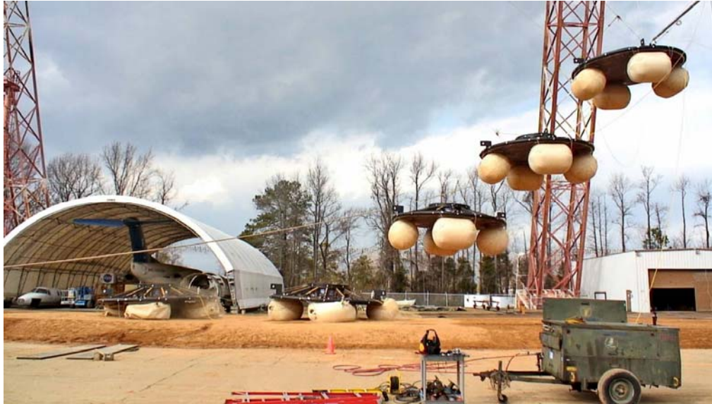
Figure 4: Time-lapse composite image of pendulum-style drop test of airbag model.
