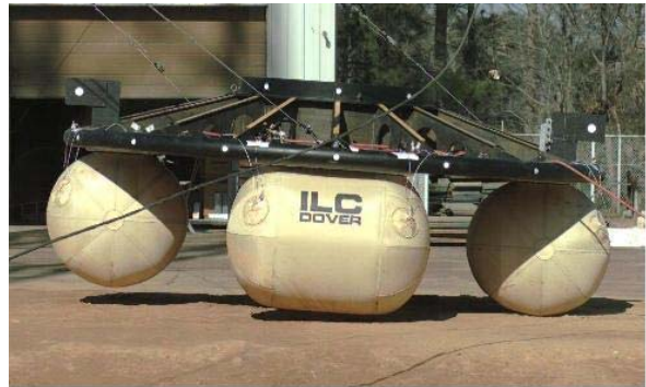
Figure 10: Single frame of high-speed (1 kHz) video showing ground impact of airbag drop model outfitted with ILC Dover airbags.
