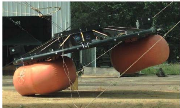
Figure 11: Single frame of high-speed (1 kHz) video showing ground impact of airbag drop model outfitted with Irvin Aerospace airbags.
