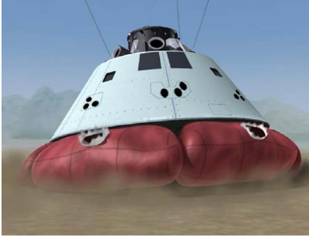
Figure 2: Artist's rendition of Orion with airbag landing attenuation system.
