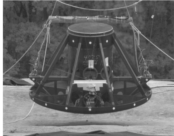
Figure 6: Second generation half-scale Orion metal shell drop model.
