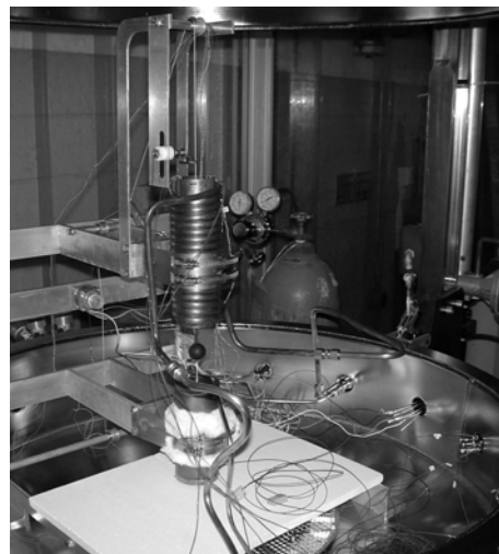
Figure 5. Heat sponge heat capacity characterization apparatus
