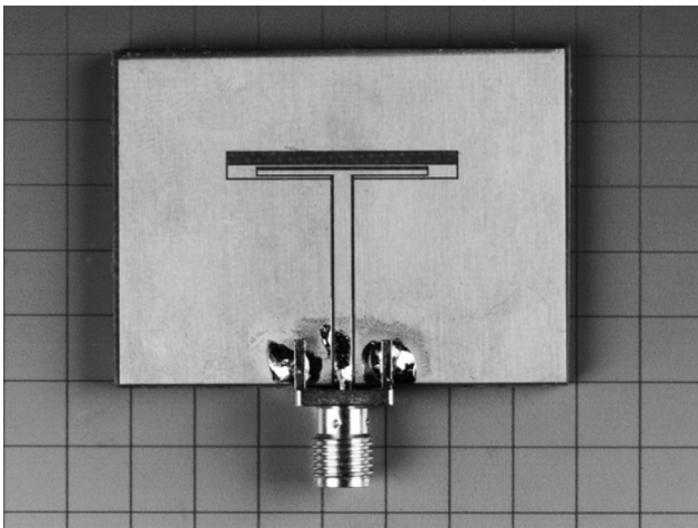
Figure 2.—Experimental setup showing the transition from the coaxial connector to the coplanar waveguide feed.
