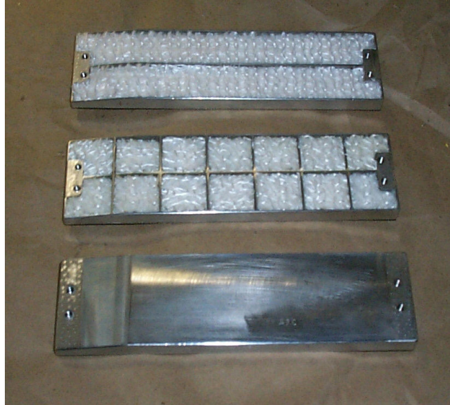
Figure 6.—Rear view of treatment trays: parallel rib (top), grid rib (middle), solid wall (bottom).
