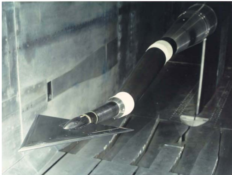
Figure 2. NASA NTF tests on the 65^\circ delta wing (Ref. 1)
