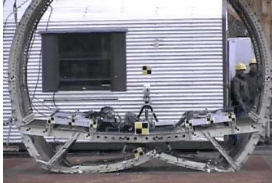
Figure 3. Photograph of deformed Fokker F28 fuselage section.
