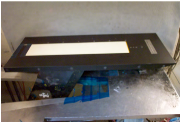
Figure 3. Baseline model with 4-inch by 18-inch ceramic inserts used in Mach 6 for T6888.
