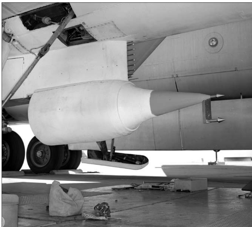
This is how the ventral stabilizer and ramjet installation looked on the morning of 3 October 1967 prior to Flight 2-53-97. The skid landing gear is extended in this photograph. (NASA)
