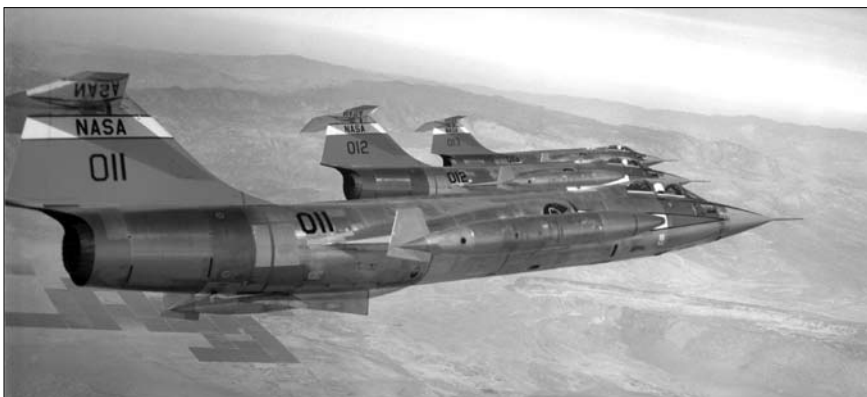
The Lockheed F-104 Starfighter was used as a chase airplane and to practice landing maneuvers. In addition to the F-104Ns owned by NASA, various F-104s from the Air Force Flight Test Center were used as needed. (NASA)
