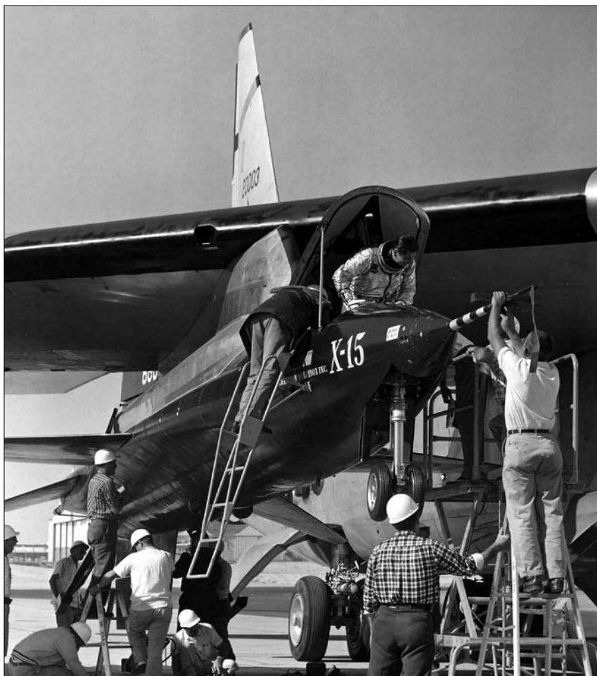
Scott Crossfield climbs out of X-15-1 after the first captive-carry flight. The X-15 landing gear had been deployed during the flight to demonstrate it would work after being cold-soaked at altitude. A member of the ground crew installs protective covers on the nose-mounted air data boom. (AFFTC History Office)
