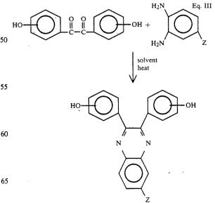
where Z=H, Cl, Br, OCH<sub>3</sub>, CH<sub>3</sub>, CH<sub>2</sub>CH<sub>3</sub>, or Ph. The catenation of the hydroxy group may be meta-meta, para-para, or para-meta.
