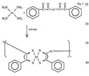
Polyphenylquinoxalines prepared from such condensations are configurationally unordered with three possible isomers distributed randomly along the polymer chain; see Hergenrother, *Encyclopedia of Polymer Science Technology*, Vol. 13, p. 55, (1988).
