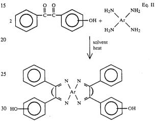
where Ar is 1,2,4,5-tetrasubstituted benzene, 3,3',- 4,4'tetrasubstituted; biphenyl, diphenylether, diphenylmethane, diphenylketone, diphenylsulfone, diphenylthioether or any appropriate bis(o-diamine) and mixtures thereof. The catenation of the hydroxy group may be meta-meta, para-para, or para-meta.
