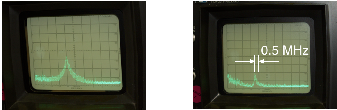
a. Magnetic harmonic response with no fluid in container. b. Magnetic harmonic response with container approximately half full
