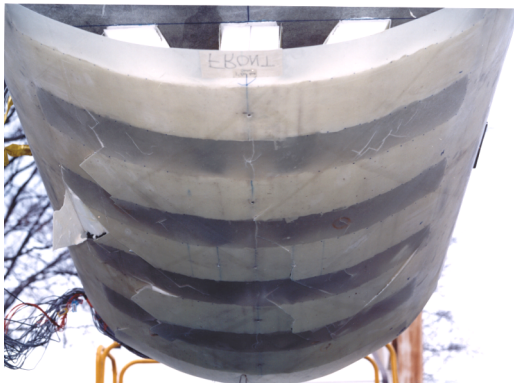
Figure 9. Bottom of fuselage showing damage. The four dark regions are areas between the foam blocks.
