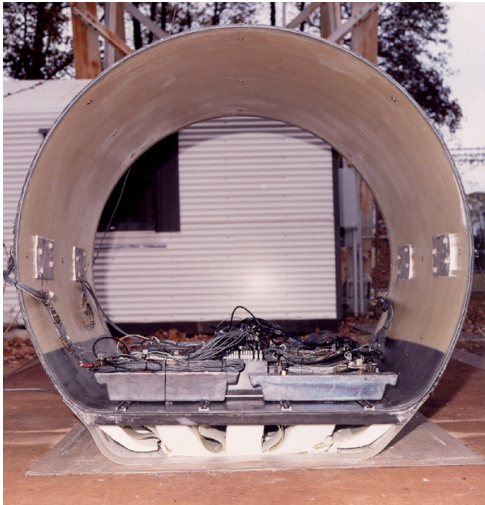
Figure 5. Post-test photo of the composite fuselage after impact onto a rigid concrete surface.
