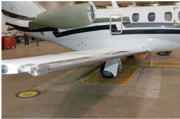
Figure 4(a).—Wing ice protection system failure case.
