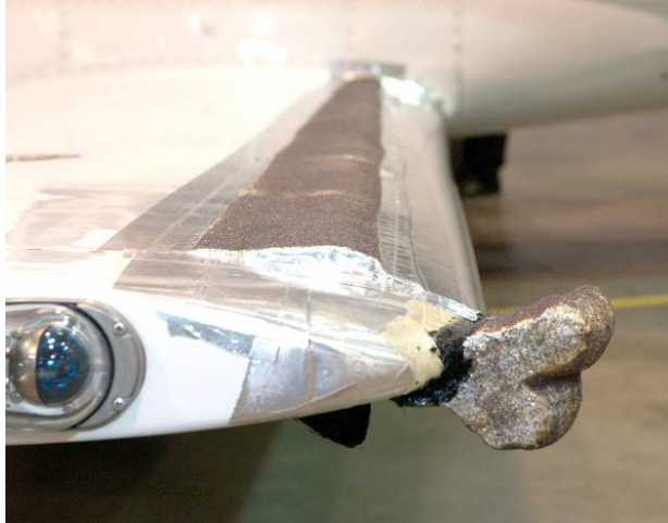
Figure 3(a).—Upper wing runback shape.
