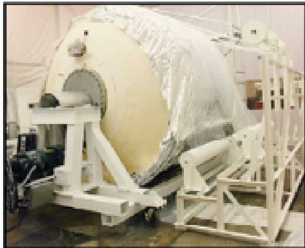
Figure 2. Application of Variable Density MLI to test tank.
