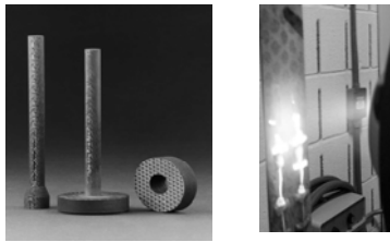
C-C Engine Valve Attachments for Sensors
