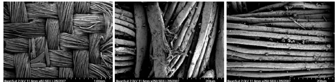
Electron micrographs from GRC showing damage to the outer layer of Alan Bean's Apollo 12 suit
