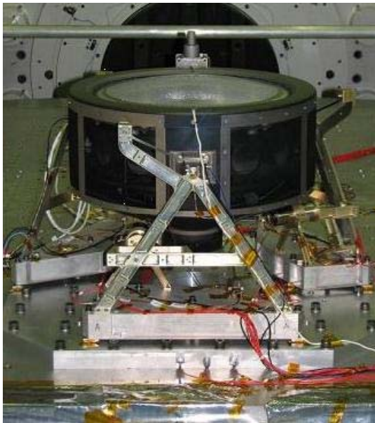
Figure 3 – PM thruster/gimbal assembly in vibration test preparations.
