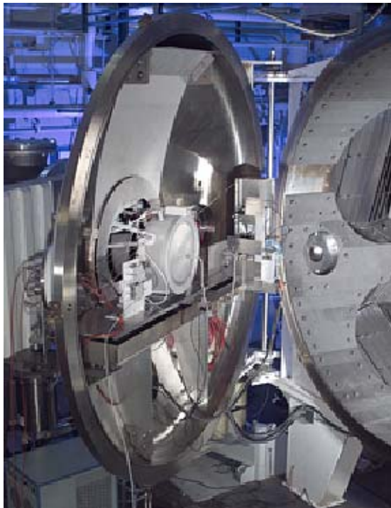
Figure 5 – NEXT thruster long duration test set-up in vacuum facility 16 at NASA GRC.
