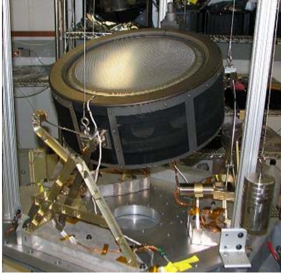
Figure 9 – NEXT gimbal during functional testing with the PM thruster.
