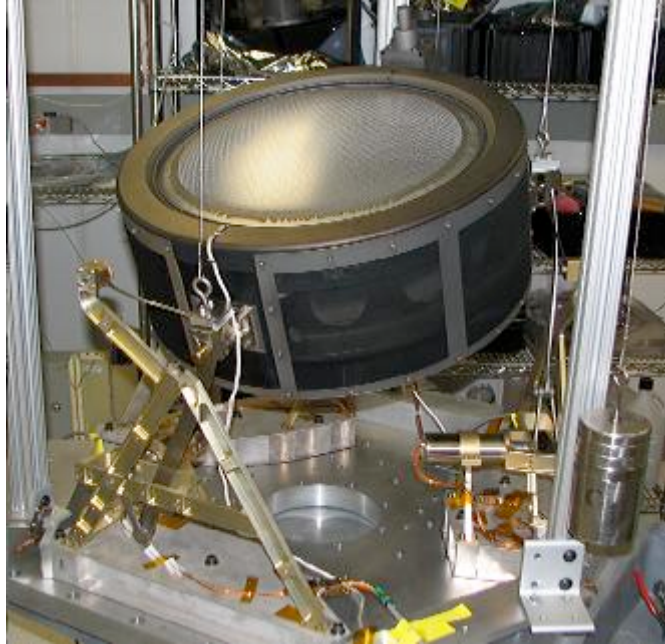
Fig. 7. Gimbal functional testing with the PM1 thruster
