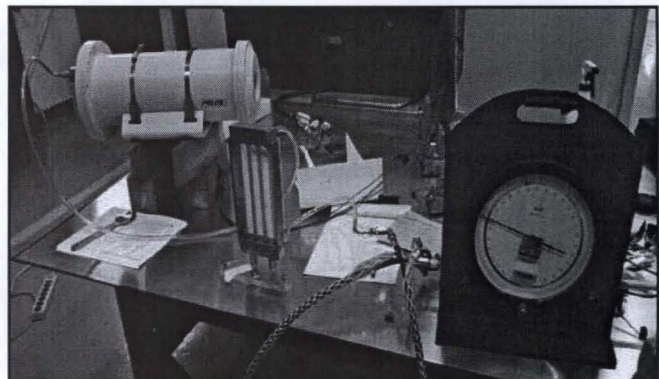
Figure 27. Pressure test with Kellum tether.
