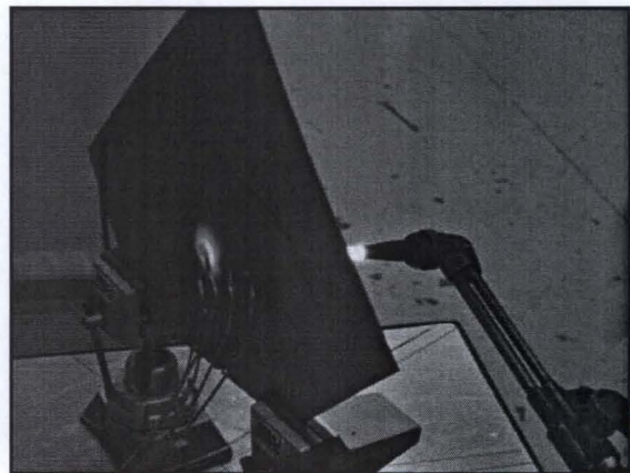
Figure 20. Heat being applied to instrumented panel.
