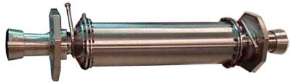
Figure 2.—Stirling convertors joined at alternators by interconnect tube.
