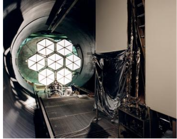
Figure 7.—Solar Dynamic Ground Test Demonstration (SD GTD) View from Solar Simulator Window.
