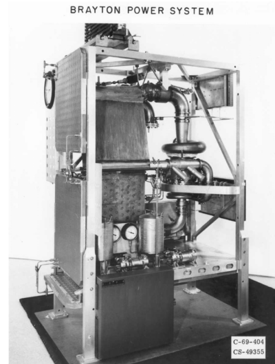
Figure 3.—BRU and BHXU in Test Rig at Lewis.
