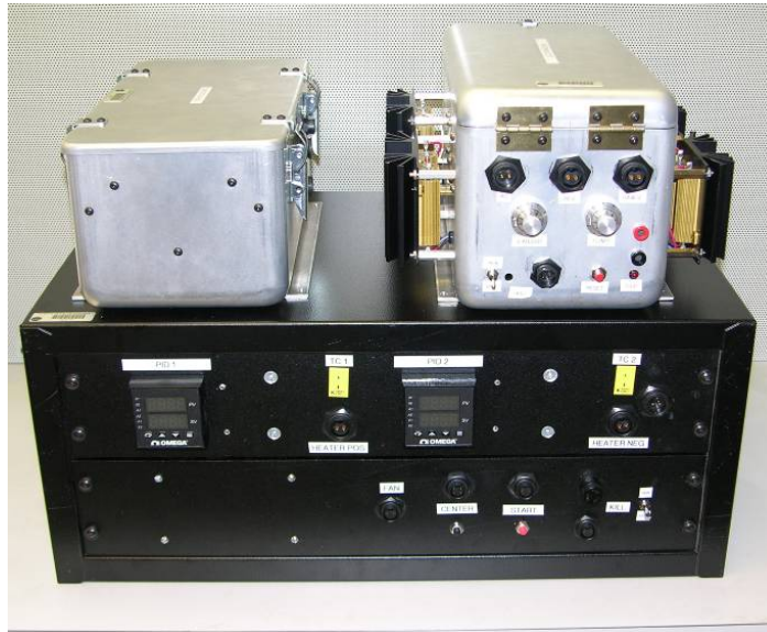
Figure 8.—ASRG simulator support equipment. Tuning capacitor bank (top left), control electronics (top right), and ground support equipment (bottom).
