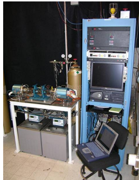
Figure 2.—Extended operation test station. A pair of ASC-0 units setup for continuous unattended operation in air.
