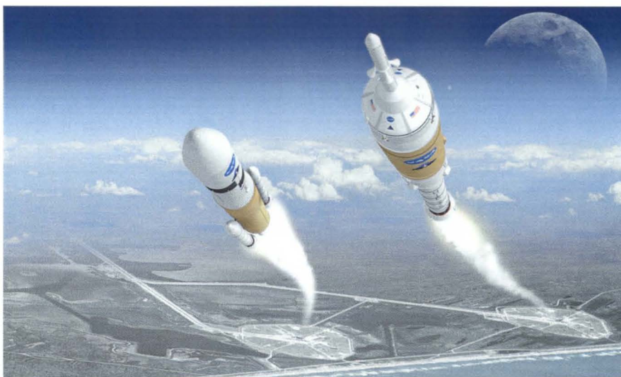
Fig. 1. Concepts of the Ares I crew launch vehicle (right) and Ares V cargo launch vehicle.
