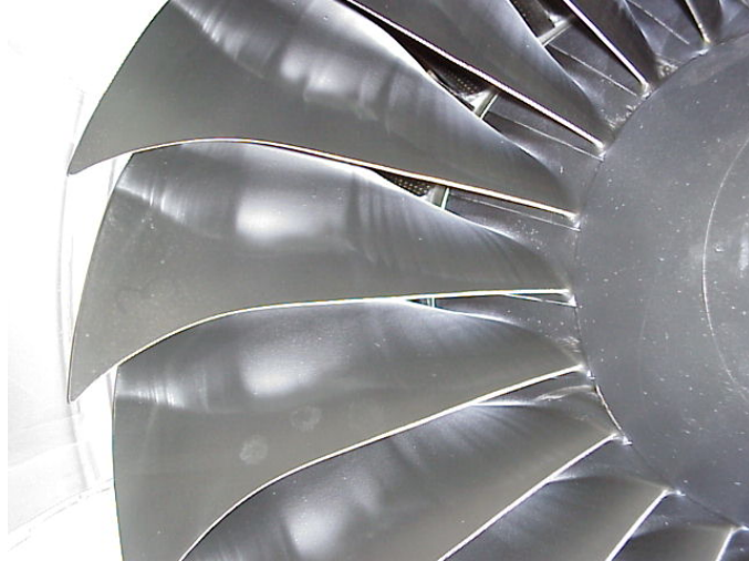
Figure 8.—Photograph of forward-swept fan blades after LDV test in which the rotor was operated at the high-speed condition (13831 rpm c ). The photo shows the build-up of LDV seed particles on the suction side of the rotor blades.
