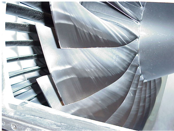
Figure 9.—Photograph of aft-swept fan blades after LDV test in which the rotor was operated at the both the mid (12500 rpm c ) and high (13831 rpm c ) speed conditions. The photo shows the build-up of LDV seed particles on the suction side of the rotor blades.
