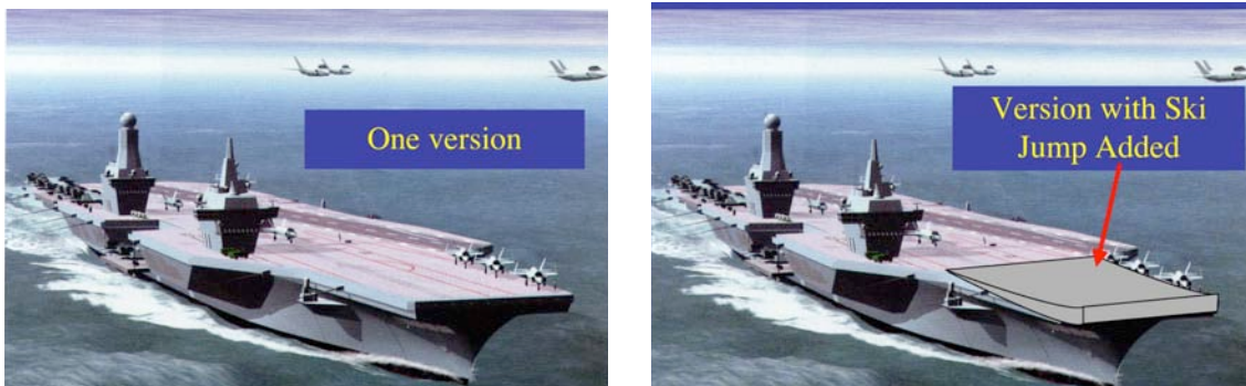
Figure 6. Proposed British aircraft carrier without [4] and with ski-jump.
