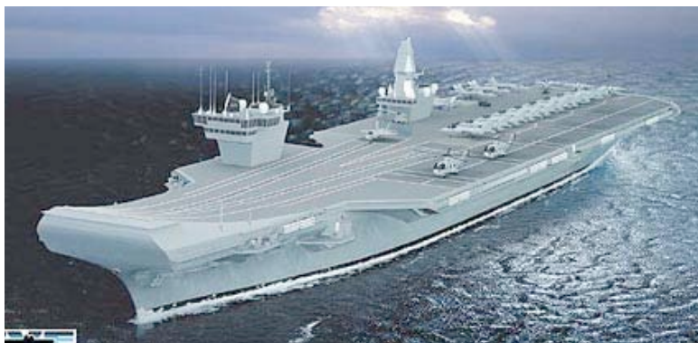
Figure 7. Alternative British aircraft carrier with ski-jump [5].
