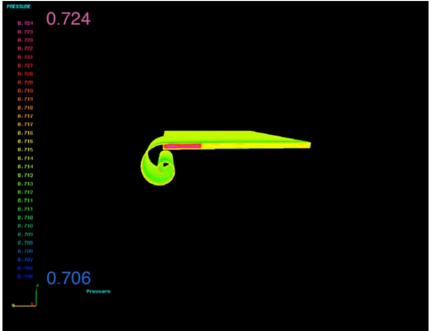
Figure 18. USM3D solution for modified CVG device mounted on flat plate at \alpha \sim 0^\circ (looking aft): C_p results.
