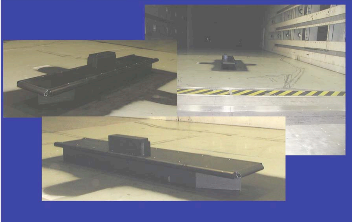
Figure 26. Three views of simplified 1/120 th scaled LHD model with devices in 14 ft by 22 ft wind-tunnel.
