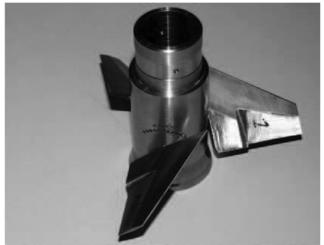
Fig. 3 Modified tailcan of the 3%-scale Hyper-X launch vehicle stack model with fin settings of 51 deg.
