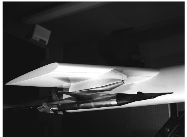
Fig. 5 Side view of the partial B-52B airplane model with the 3%-scale Hyper-X launch vehicle stack model.
