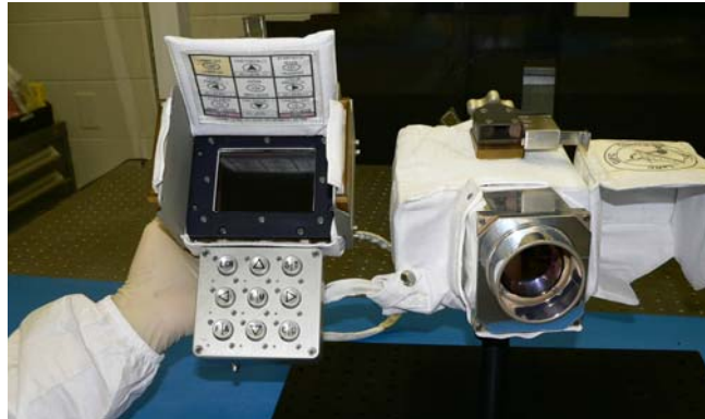
Figure 1. Photograph of EVA IR Camera Flight Unit. The camera consists of two major components: the camera body with the germanium infrared detector, battery, memory, and flash drive, and the Remote Control Unit (RCU) containing the LCD screen and control buttons.
