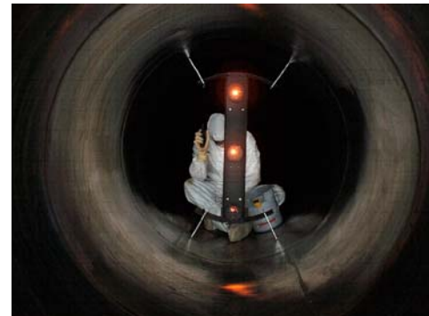
Figure 11. DART target during 500 meter vacuum tunnel testing
