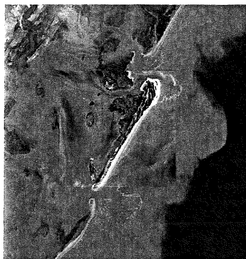
Figure 1. Multisensor registration of ETM+ at 30m (surround) to IKONOS at 1m (inset)
